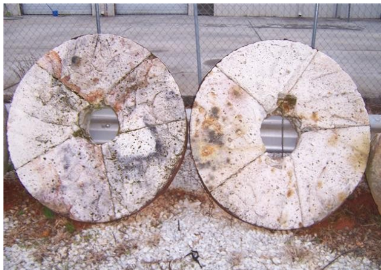
Typical French millstones. Each stone is made of several pieces of French burrstone which have been cut and pieced together then held by an iron band.
